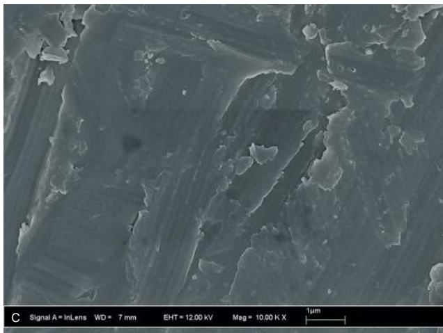
Fig 3a–c Scanning electron micrograph images showing the roughness of the cage surface imparted by PROTI 360°™ Titanium Integrated Technology (b) compared to PEEK (a) and smooth titanium (c).
